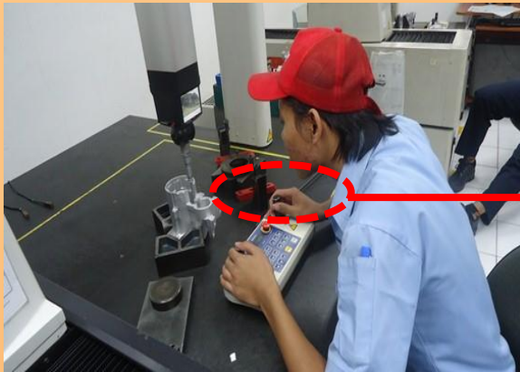
Inspector Measuring By CMM at Diameter Lever area for verification when found abnormality condition.
