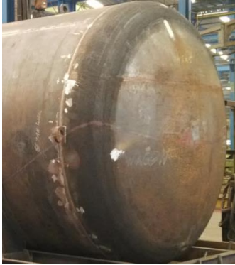
Figure 2.17 Welding The Disc End
