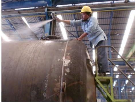
Figure 2.20 Air Pressure Test & Final Check
