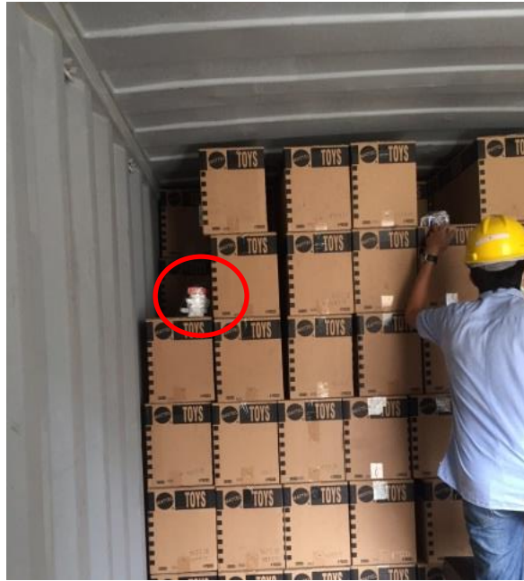
Figure 4.7 Temperature Data Loggers Inside Container
