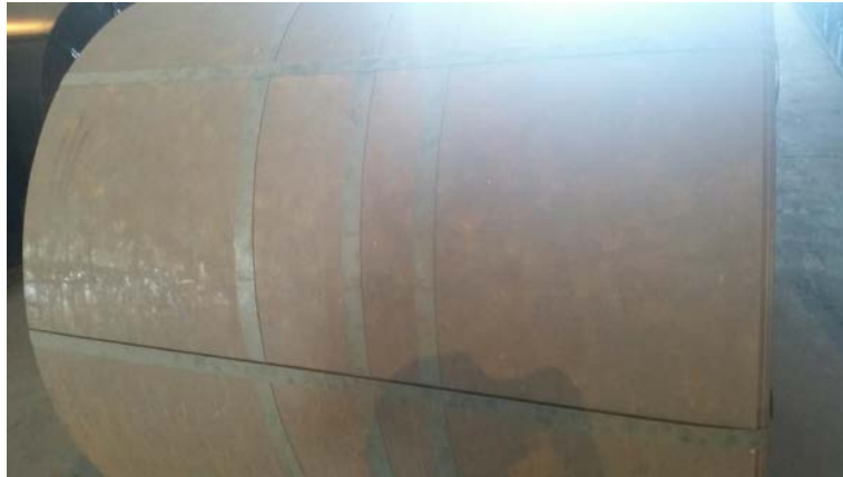
Figure 4.16 Heavy Rusting Defect
