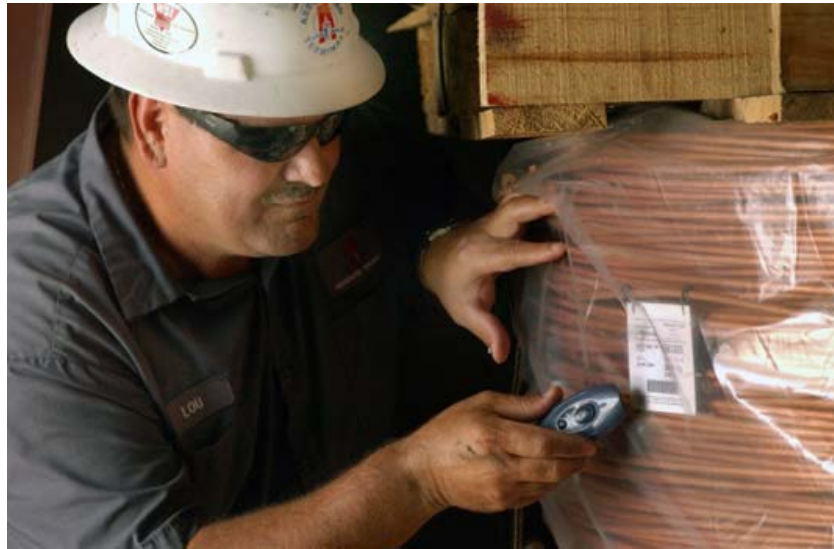
Figure 4.32 Barcode Use on Finished Products
