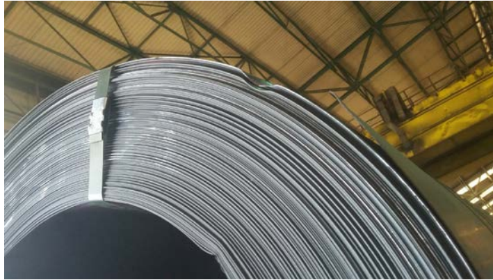
Source: Courtesy of PT. X Figure 4.10 Edge Fold Defect
