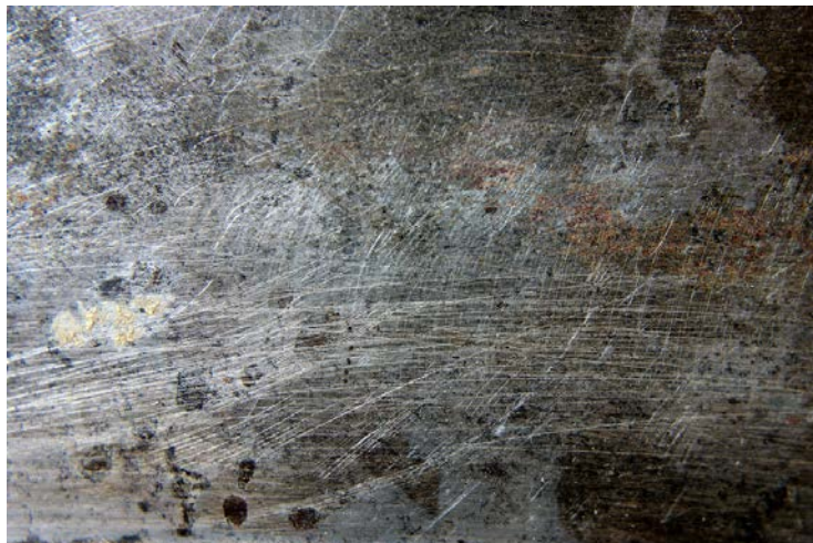
Figure 4.9 Scratched Surface of Hot Rolled Coil
