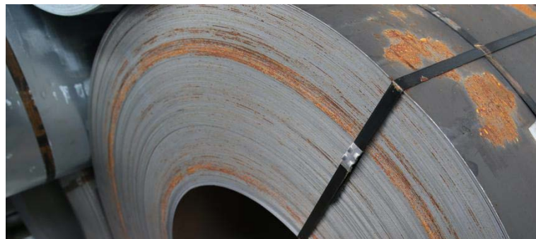
Source: Courtesy of PT. X Figure 4.15 Mild Rusting Defect
