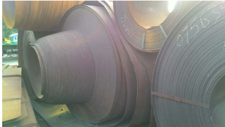
Source: Courtesy of PT. X Figure 4.14 Telescope Defect
