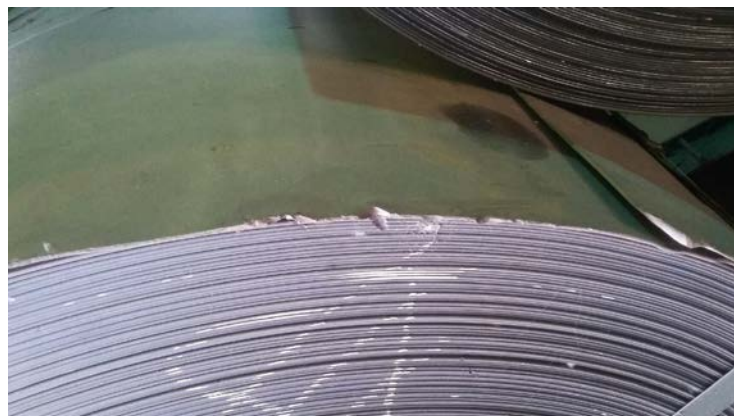
Source: Courtesy of PT. X Figure 4.11 Edge Crack Defect
