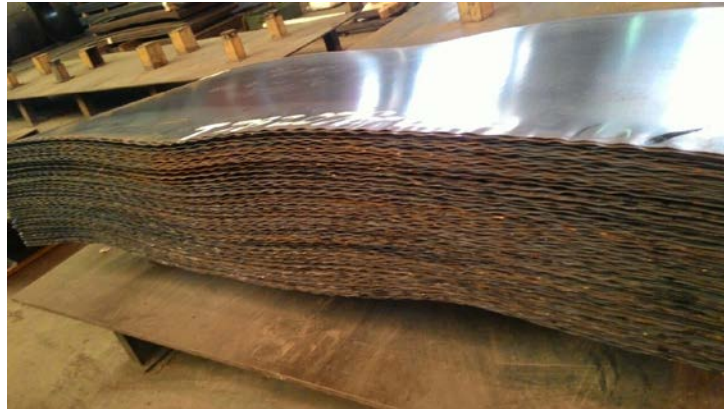
Source: Courtesy of PT. X Figure 4.13 Wavy Defect
