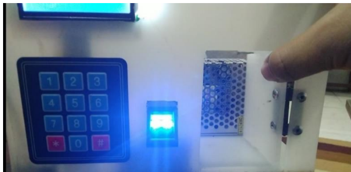
Figure 4.5 Prototype Testing Solenoid Door Lock.
