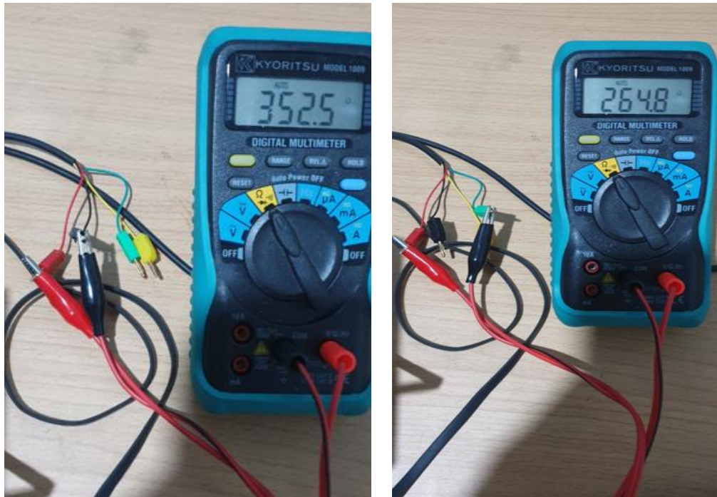
Gambar 7: Nilai tahanan strain gauge
