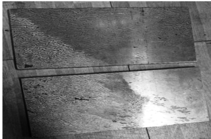
FIGURE 3. Specimen of Al 5083 alloy before welding.
