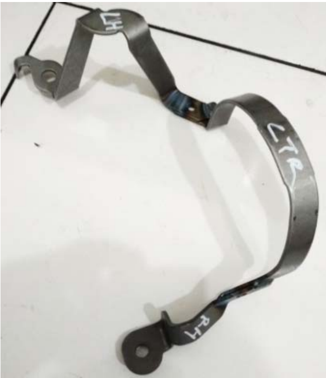
Fig. 5. Propeller Shaft Guard All Joint in one Part [5].
