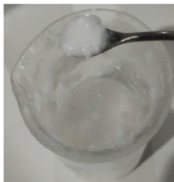
Figure 4. SiO 2 deposits formed after acidification
