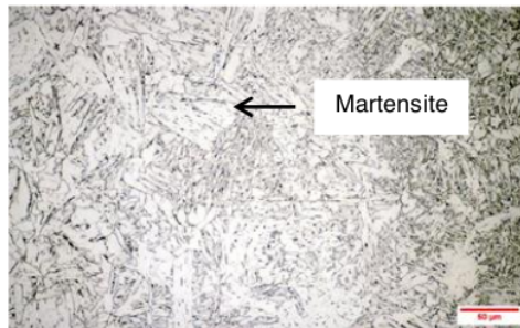
Figure 5. Microstructure at HAZ without WPS
