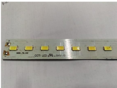
Gambar 3. LED SMD Osram Duris E3 (3.0x1.4mm).
