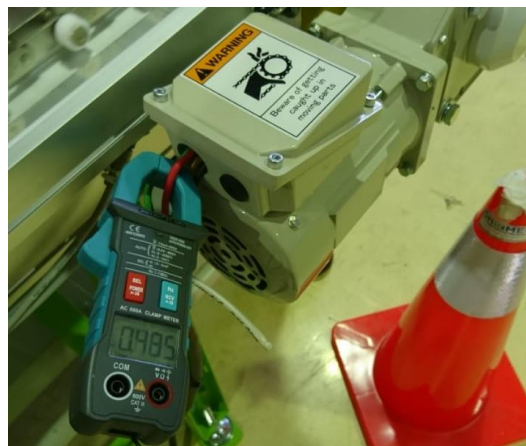
Figure 4. Direct measuring of the load current
